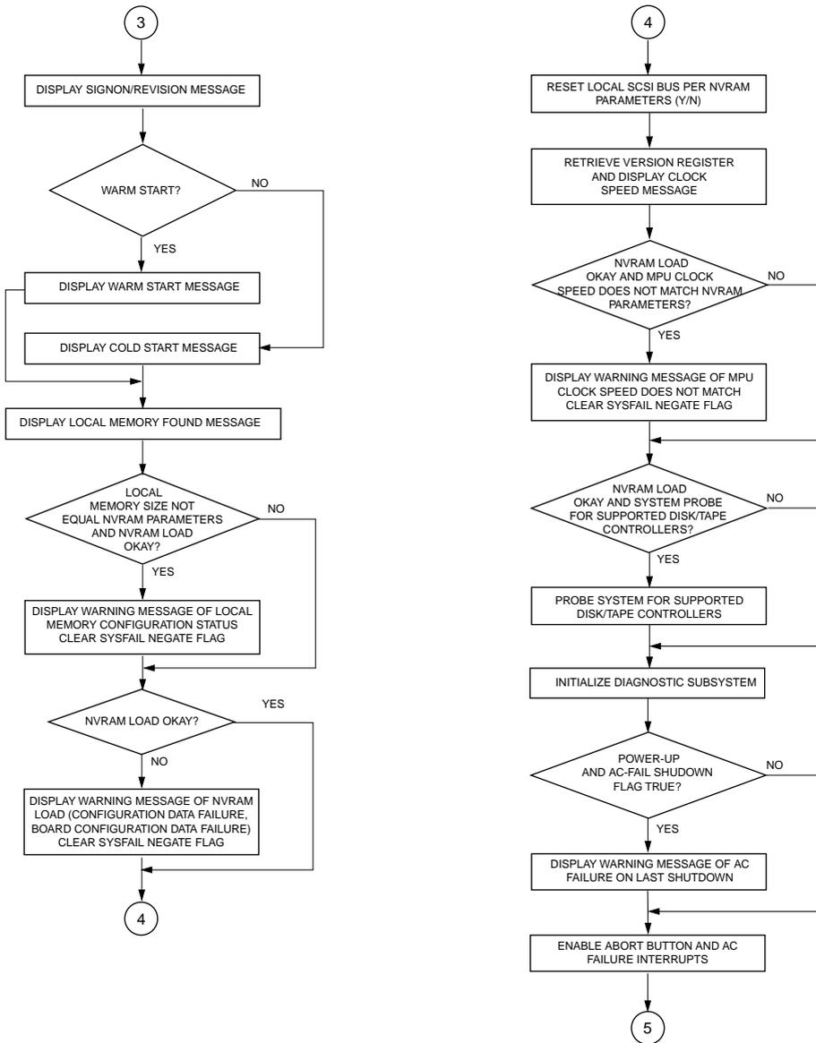
**Figure 1-1. 162Bug Start-up Flow (Sheet 2 of 3)**
