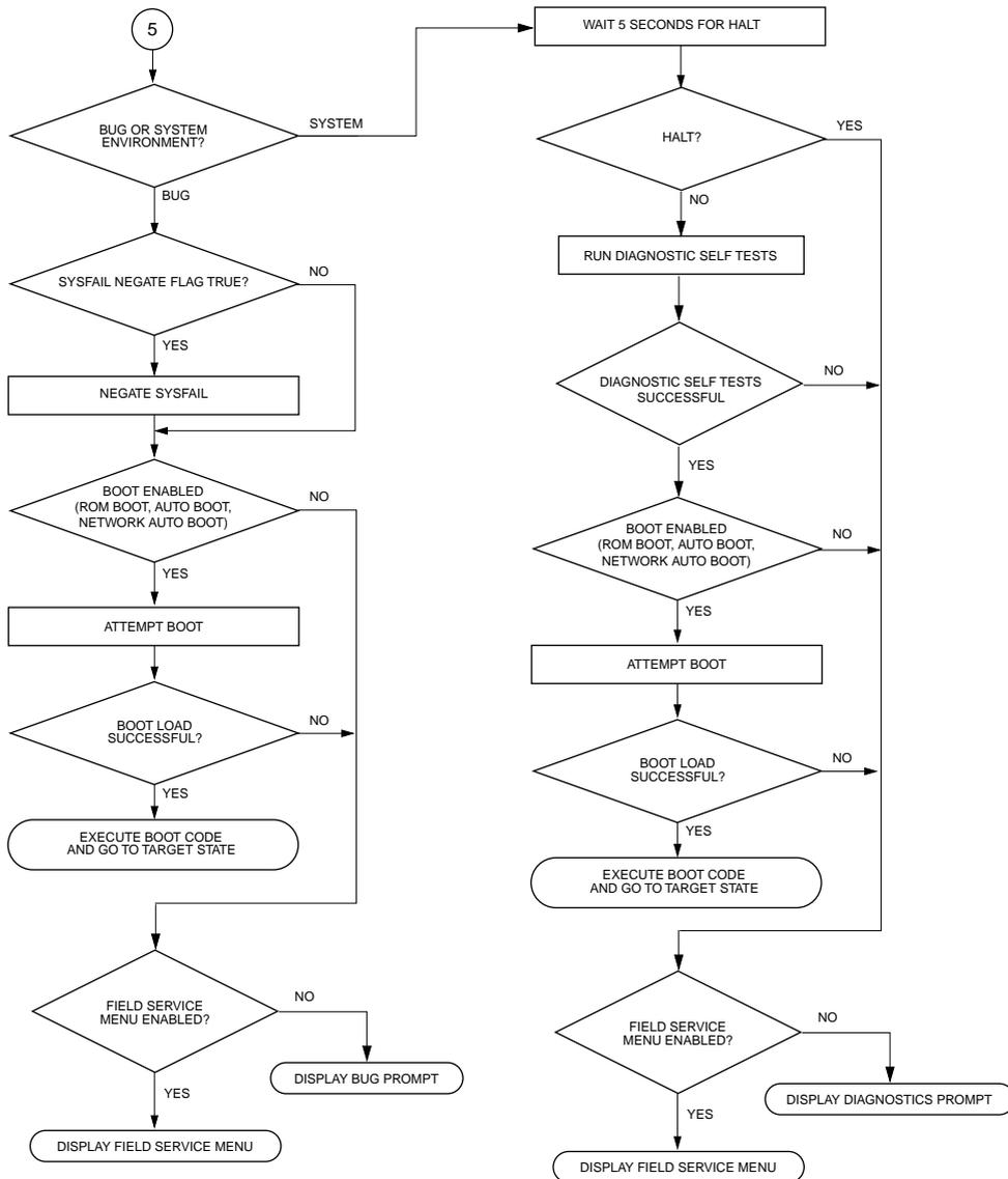
Figure 1-1. 162Bug Start-up Flow (Sheet 3 of 3)
