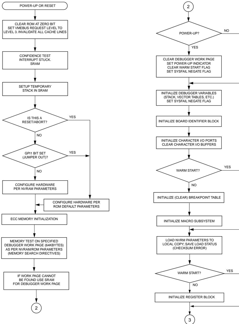
Figure 1-1. 162Bug Start-up Flow (Sheet 1 of 3)
